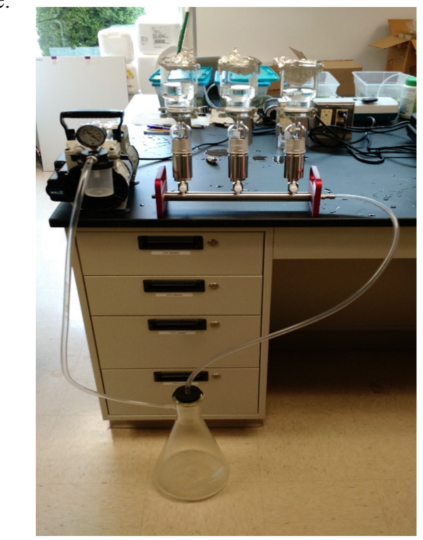
Figure 11: Solid-phase extraction equipment. This set up was used to extract and concentrate chemicals from natural samples.
