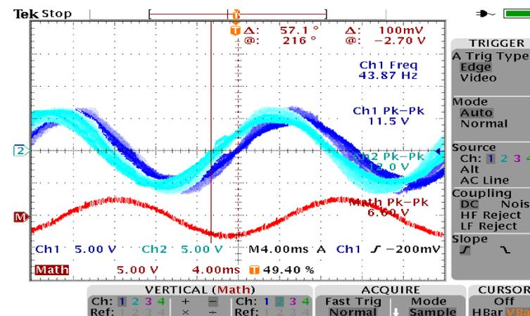
Ch1: One side of the third resistor in a six resistor divider between the BLK & RED phase outputs
