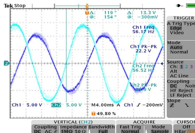
Ch1: Outside of the first resistor in a six resistor divider between the BLK & RED phase outputs
