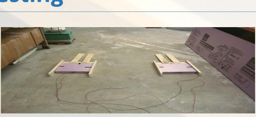
Field Testing Was Performed at Buckman Hall By The Docking Area. The Following Vehicle Model Drove Over built Ramp Making A Stop And Go Simulation.
