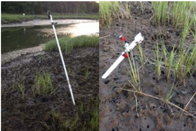
Figure 3 Camera array, right: GoPro with red flash lights, left: infrared camcorder with infrared lamps
